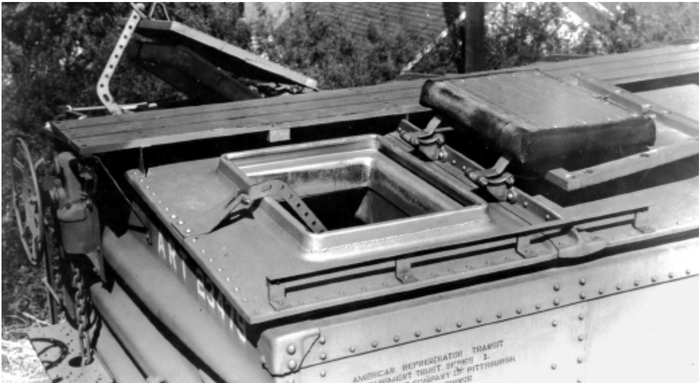
APPLICATION OF GUARD ANGLES TO ROOF.
