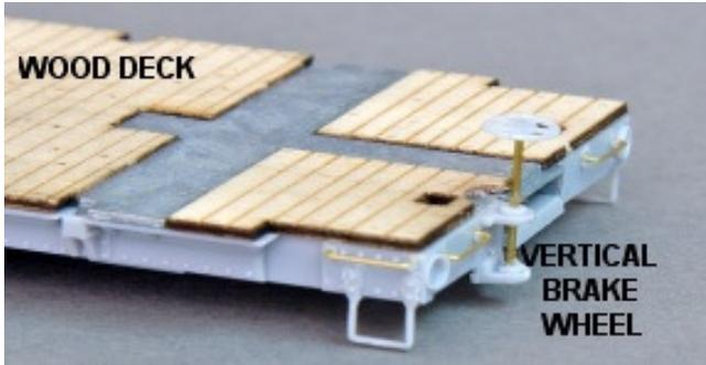
Step 15. If assembling the car with the bulkheads, the four corner wood parts are smaller, and are located against the raised corners at the bolsters. Glue the laser cut wood deck parts to the top of the weight. Refer to the BULK HEAD ASSEMBLY instructions to assemble the bulkheads.
