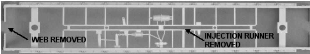
Step 3. Remove any flash from the underframe, and separate it from its sprue. Test fit the underframe into the body. Note that the cross bearers of the underframe have molded notches to fit over the connections of the brake system.
