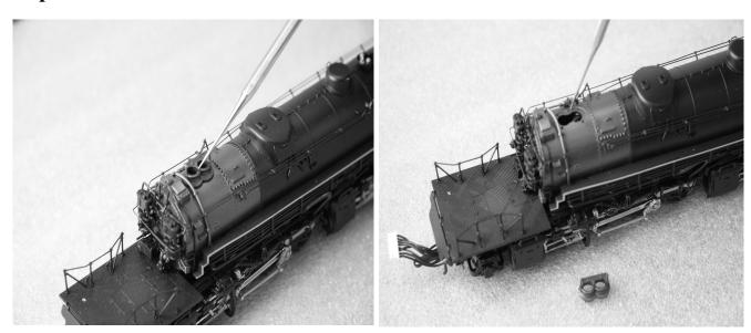
Remove the smoke stack so you can access the capacitor. The smoke stack is press fit in place but may require a little effort to remove.
