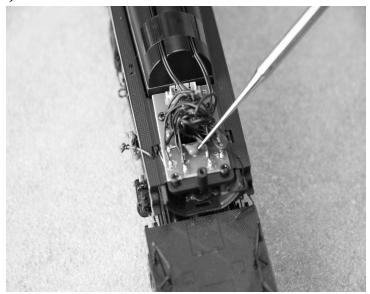
This image shows the capacitor that is going to be removed. The boiler has been removed in this image so you can see the capacitor. The capacitor is orange/yellow in color.
