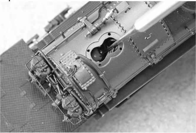
From the image above you can see the capacitor through the smoke stack opening. Using either a flat bladed knife, or a pair of long nose cutters, reach in the smoke stack and cut one end of the capacitor.
