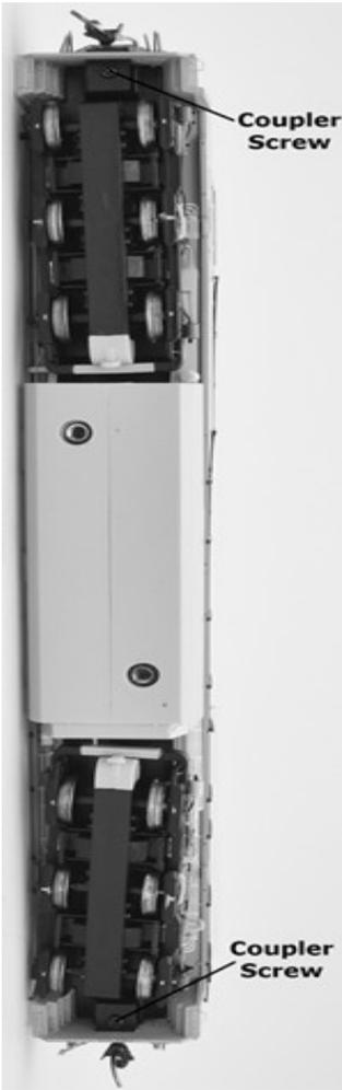
2. Pull upward on the shell using a steady controlled pressure. Be gentle and take your time to avoid damaging any of the locomotive details. Once the die-cast chassis begins to slide out from the shell, take care to guide the front and rear portions evenly. DO NOT wedge the chassis against the shell.
