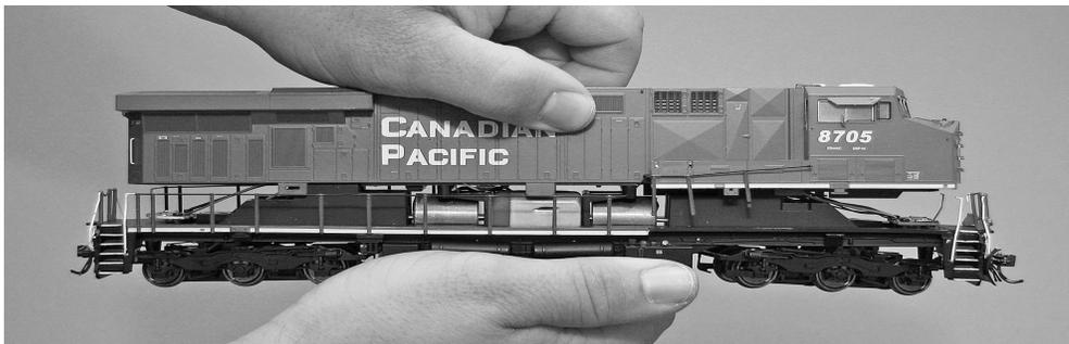
2. To remove the shell, firmly grip the fuel tank area and the center area of the body. Gently rock the shell side to side to release the holding tabs and lift straight up. Watch that the handrails do not get caught on the body deck or cab while being lifted off.
