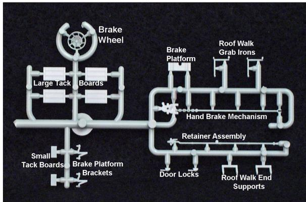
Step 11. Attach the small tack boards to the lower left of the doors. Attach the large tack boards to the lower right of the later Youngstown doors. If the original six-rib doors have been used, the large tack board is attached to the side of the car, to the left of the door, between the fourth and fifth rib from the side sill.
