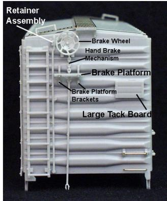
Step 17. Attach the two wire grab irons to the lower right of the ends.
