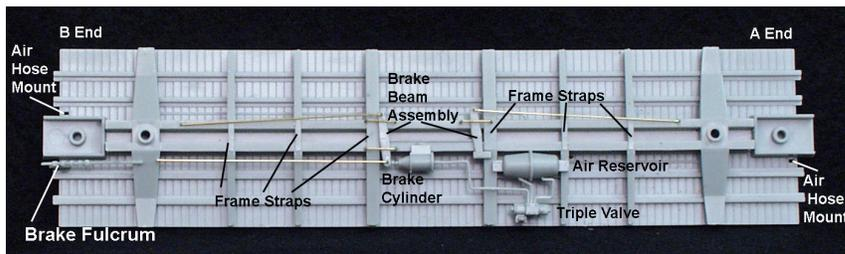
Step 2. Remove the six frame straps from their sprue. Attach the one wide strap which has a small hole in the recess at the wide center cross bearer that also has a small hole. Attach the other wide strap and the four narrow straps into the other recessed locators between the cross bearers of the frame.
