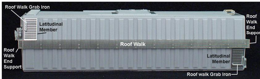
Step 19. Attach the roof walk grab irons to the latitudinal members, and the roof walk end supports in the locator holes provided at the top of the end. Enlarge the locator holes for the roof walk end supports with a no. 70 (.028 in. dia.) drill. The body assembly can be painted now.
