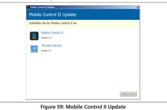
Now connect the meanwhile active Mobile Control II with a USB port of your computer. The device must be detected automatically. The software offers the update of both Apps automatically, which are provided by ESU for the Mobile Control II.
