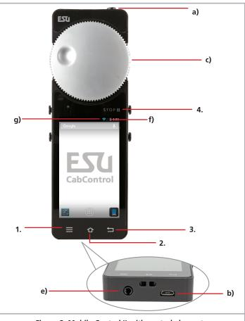
Figure 2: Mobile Control II with control elements
