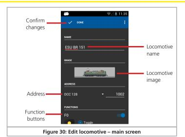
Once you have confirmed all changes press the "Save" button. For saving all changes press the "Return" button at the bottom right of the touch screen. If you do not wish to save any changes, press the menu button at the bottom left and select "Discard changes".
