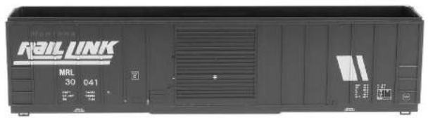
Montana Rail Link - Single Door - ACF Non-terminating Ends Date: BLT 7-84
